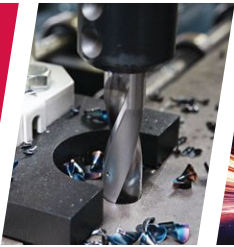
CARBIDE DRILLING 5 SECONDS PER HOLE IN 1" MATERIAL
